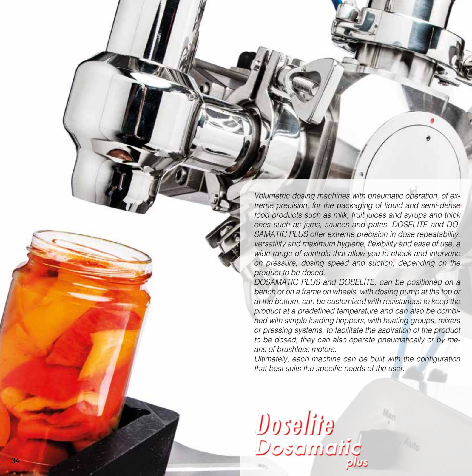
Volumetric dosing machines with pneumatic operation, of extreme precision, for the packaging of liquid and semi-dense food products such as milk, fruit juices and syrups and thick ones such as jams, sauces and pastes. DOSELITE and DOSAMATIC PLUS offer extreme precision in dose repeatability, versatility and maximum hygiene, flexibility and ease of use, a wide range of controls that allow you to check and intervene on pressure, dosing speed and suction, depending on the product to be dosed.
