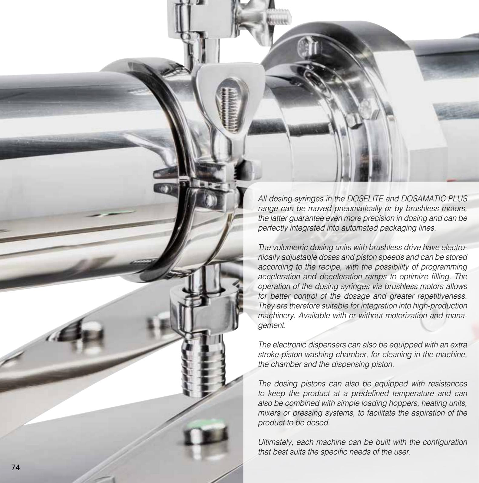
*All dosing syringes in the DOSELITE and DOSAMATIC PLUS range can be moved pneumatically or by brushless motors, the latter guarantee even more precision in dosing and can be perfectly integrated into automated packaging lines.*
